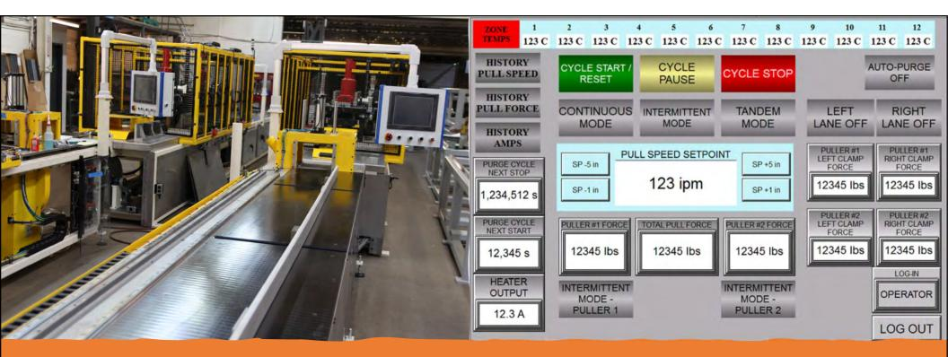
7. Control System Modern pultrusion systems are equipped with automated control systems that monitor and regulate various parameters, such as pulling speed, clamping force, and temperature (heater zones). These controls ensure consistent quality in the final product.
