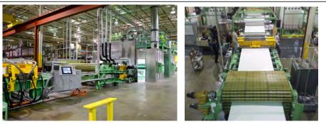
Kent Pultrusion supplied one of the largest Flat Panel Composite Pultrusion Lines in the world, processing 10 feet wide by 2"-4" thick products for the **transportation** industry.
