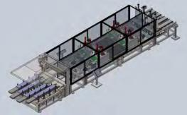
**Four Lanes -** Mechanical ability to tie lanes together for potential future operations as well as the ability to operate as one single, large, wide lane.
