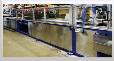
DESIGNED TO ACCOMMODATE INCREASED POWER NEEDS FOR LARGER STRUCTURAL PROFILES, THE SERVOPUL 2000 SERIES IS CUSTOMIZED TO PROVIDE MORE PULLING AND CLAMPING FORCE ALONG WITH ADDED PULLING WINDOW WIDTH AND SUPER STRUCTURAL SUPPORT FOR THE DIE.
